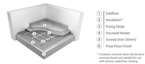
Option 2 - Wire Laid directly onto concrete pad For use where the concrete base is less than 100mm thick and insulated.
