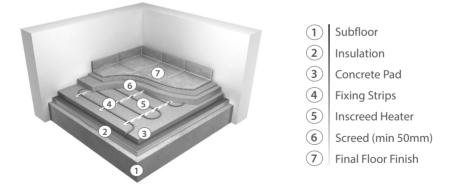
While it is acceptable to lay the heating element directly onto an insulated concrete base, insulation directly below the heater will improve the efficiency of the system. Ensure that the levels of insulation will meet your heating requirements.
